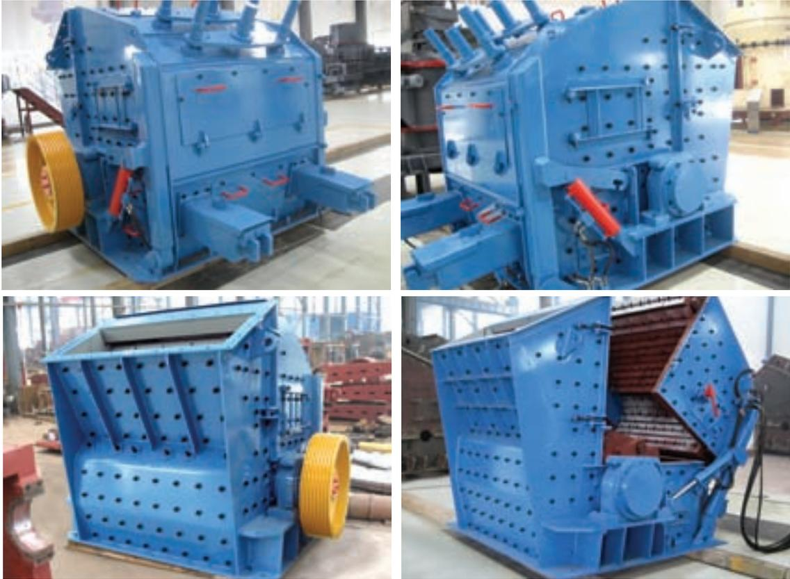
**PFW** Hydraulic impact crusher features heavy duty rotor design, unique hammer locking system, interchangeable wearing parts, and easy maintenance.
