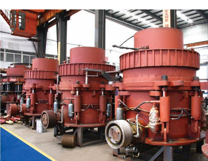
Hydraulic Cone Crusher adopts computer optimization design to speed up main shaft speed. The unique crushing chamber replace system can quickly replace components in crushing chamber to meet different size requirement.
